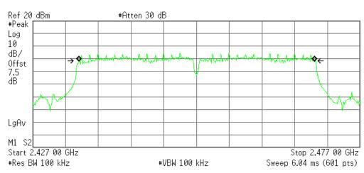
Occupied Bandwidth 35,9006 MHz Occ BW % Pwr 99.00 % x dB -6.00 dB
