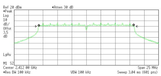
Occupied Bandwidth 16.3754 MHz Occ BW % Pwr 99.00 % x dB -6.00 dB
