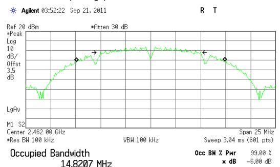
Transmit Freq Error 12.092 kHz x dB Bandwidth 9.770 MHz
