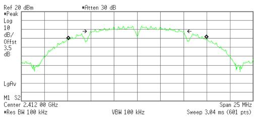
Occupied Bandwidth 14.8438 MHz Occ BW % Pwr 99.00 % x dB -6.00 dB
