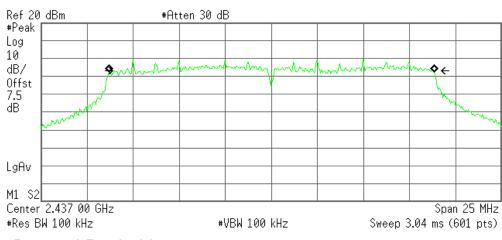
Occupied Bandwidth 17.6017 MHz Occ BW % Pwr 99.00 % x dB -6.00 dB
