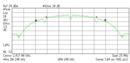
Occupied Bandwidth 14.8094 MHz Occ BW % Pwr 99.00 % x dB -6.00 dB
