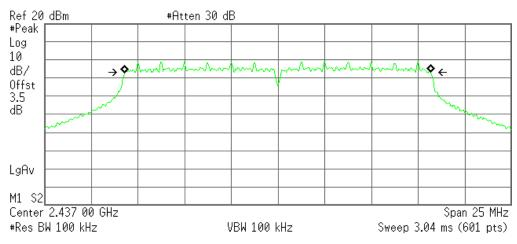
Occupied Bandwidth 16.3716 MHz Occ BW % Pwr 99.00 % x dB -6.00 dB
