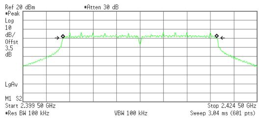
Occupied Bandwidth 16.3759 MHz Occ BW % Pwr 99.00 % x dB -6.00 dB
