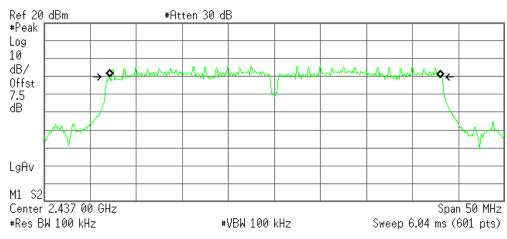
Occupied Bandwidth 35.8699 MHz Occ BW % Pwr 99.00 % x dB -6.00 dB
