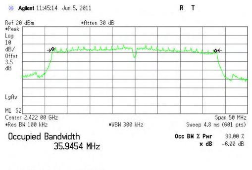
Transmit Freq Error -171.505 kHz x dB Bandwidth 35.191 MHz
