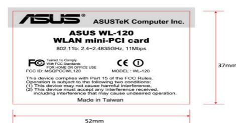
The FCC ID and DoC Label will be placed on the equipment as shown in the photograph below.
