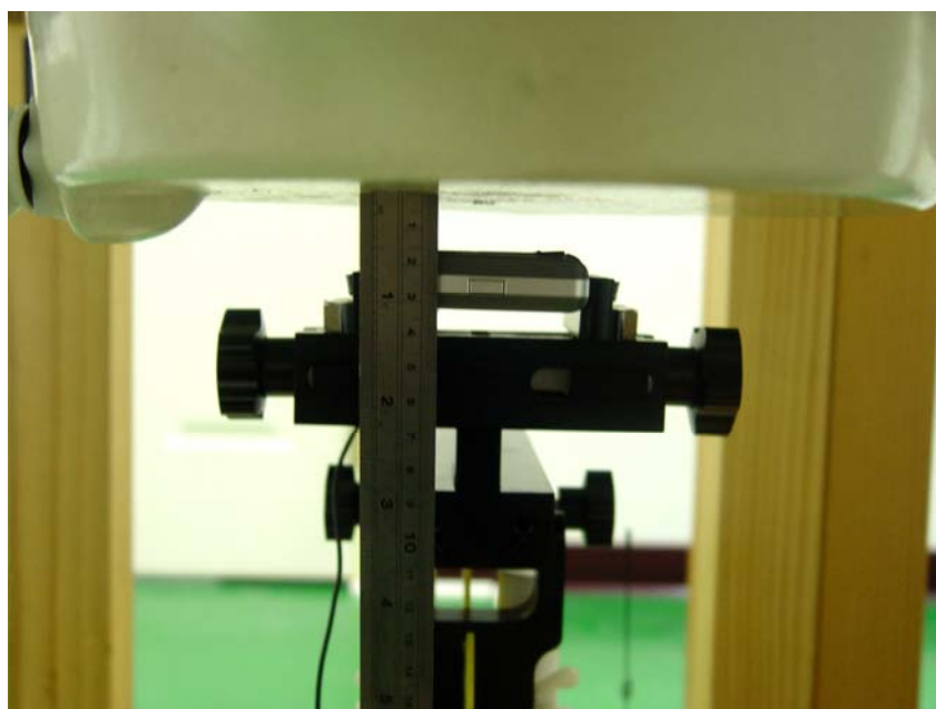
Fig. 9.8 Keypad Down with 1.5cm Gap
