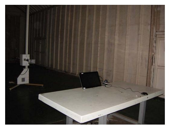
Back View of Radiated Test (Horn)
