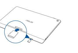
NOTE: The memory card slot supports microSD, microSDHC, and microSDXC card formats.
