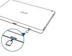
NOTE: The memory card slot supports microSD, microSDHC, and microSDXC card formats.
