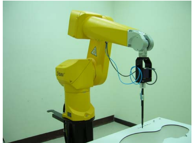
Fig. 5.2 Probe setup on robot
