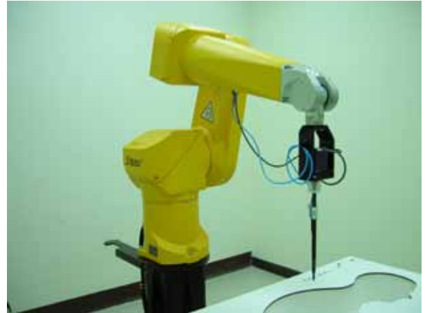
Fig. 5.2 Probe setup on robot
