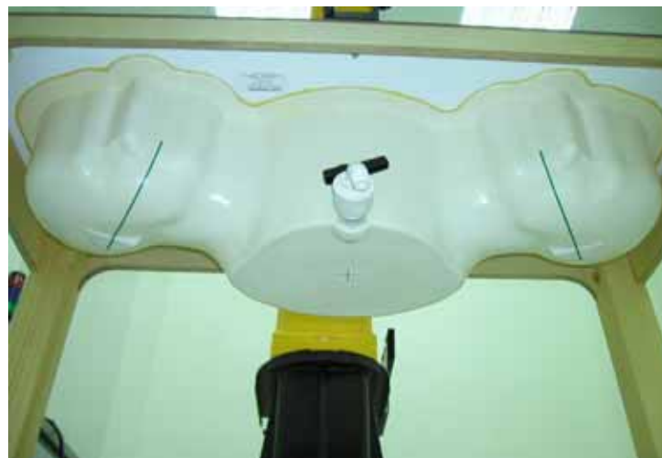
Fig. 5.4 Bottom view of twin phantom
