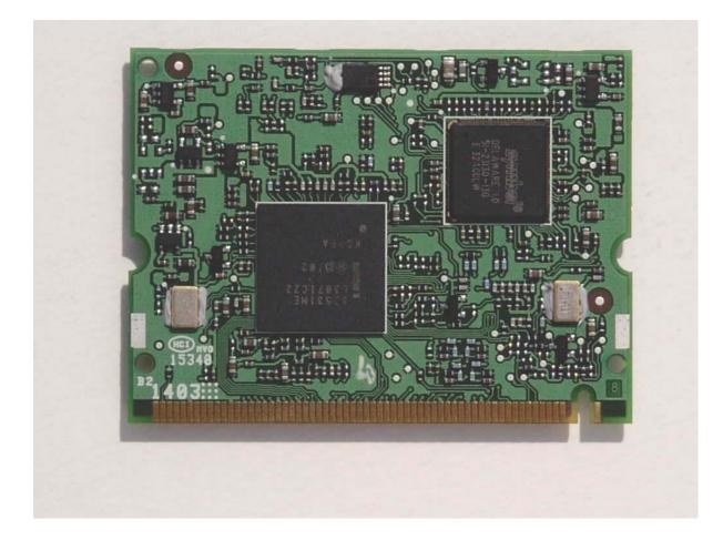
**Bottom View of the WLAN Transmitter** "Insulation Removed"
