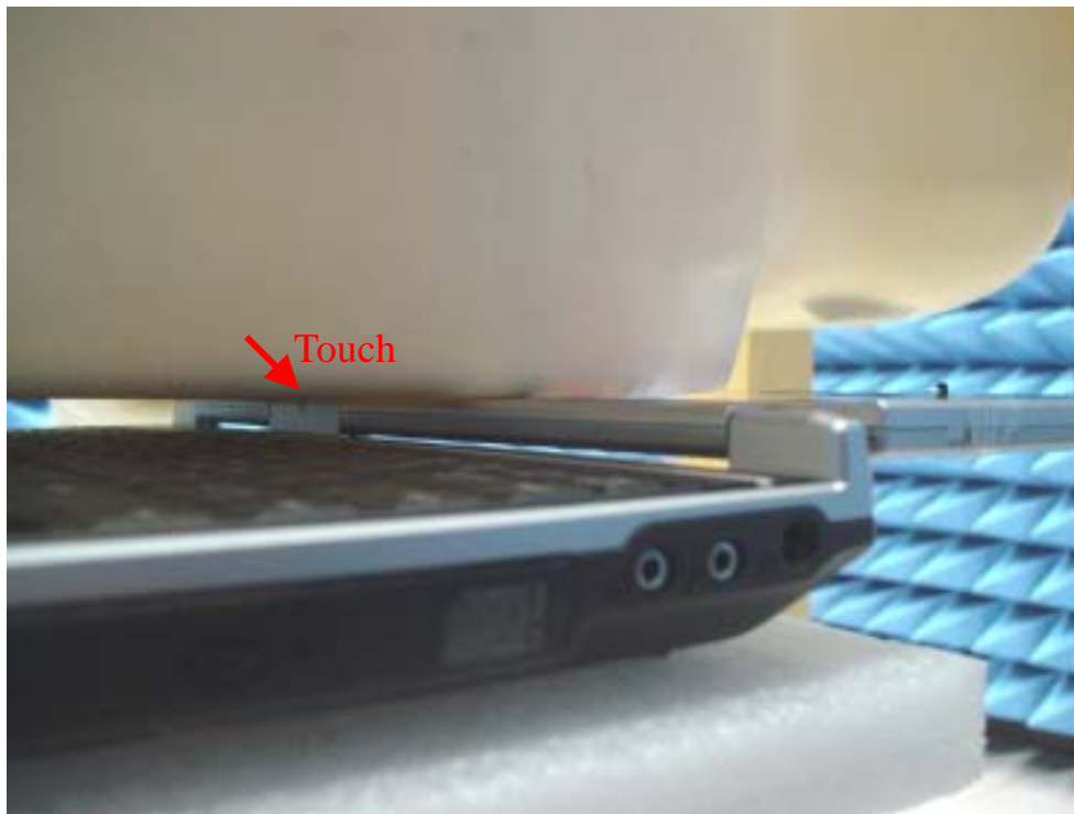
Fig.6 Photograph of the LCD panel of EUT contact to the flat phantom. The transmitted antenna of the EUT located under the reference point of the flat phantom, Spacing between EUT and phantom - In contact (0 cm)
