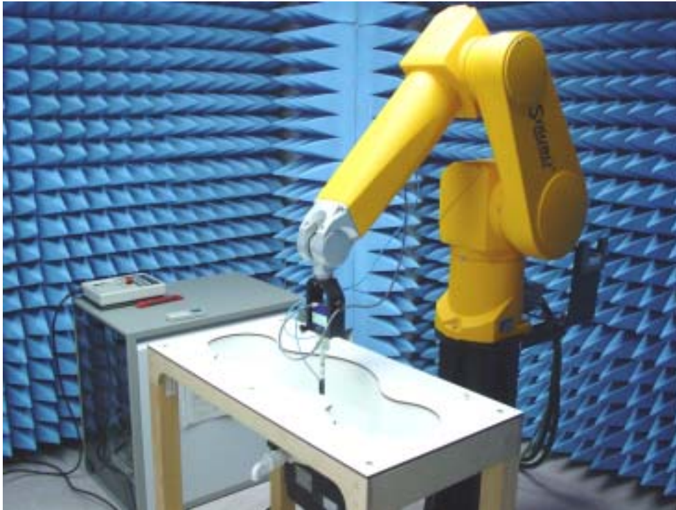
Fig.1 Photograph of the SAR measurement System
