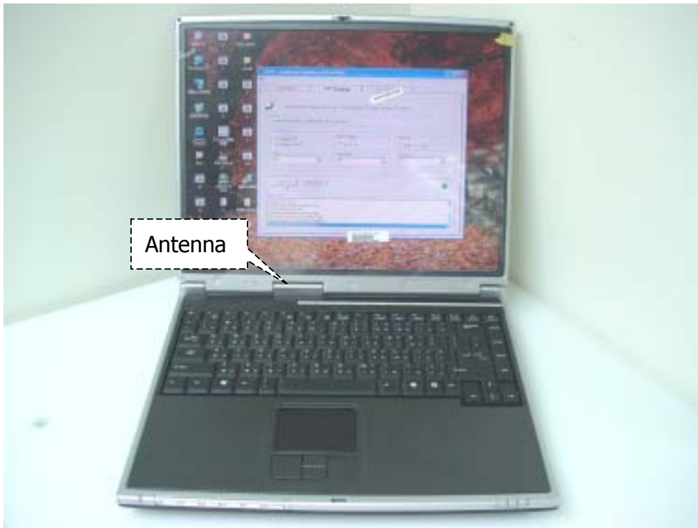
Fig.9 Antenna Position of EUT
