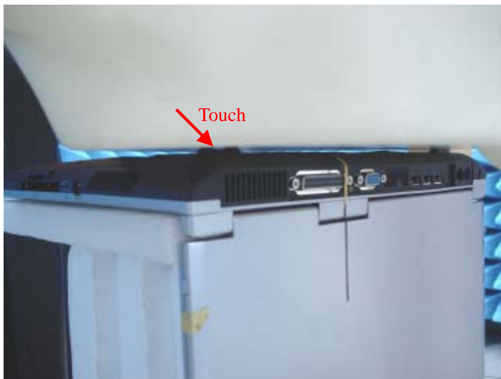
Fig.4 Photograph of the Bottom face of the EUT is paralleled with flat phantom. Spacing between EUT and phantom - In contact (0 cm)
