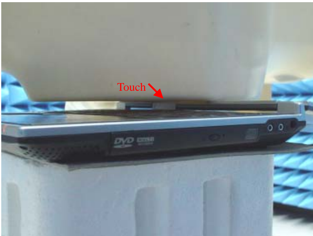
Fig.4 Photograph of the LCD panel of EUT contact to the flat phantom. The transmitted antenna of the EUT located under the reference point of the flat phantom, Spacing between EUT and phantom - In contact (0 cm)
