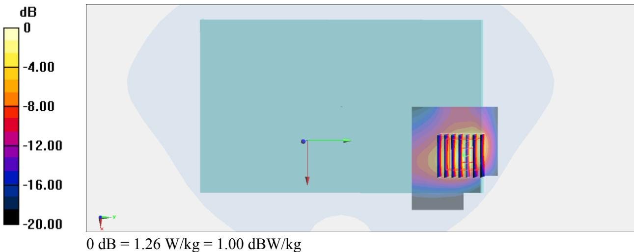
**#02\_WLAN2.4G\_802.11b 1Mbps\_Bottom Face\_0cm\_Ch1****DUT: 340938**
