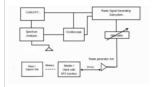
The test transmission will always be from the Master Device to the Client Device. While the Client device is set up to associate with the Master device and play the MPEG file (6  $\frac{1}{2}$  Magic Hours) from Master device, the designated MPEG test file and instructions are located at: http://ntiacsd.ntia.doc.gov/dfs/.
