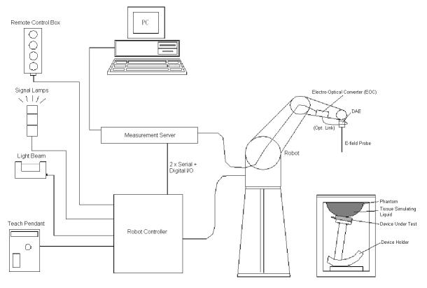
Fig-3.1 DASY System Setup
