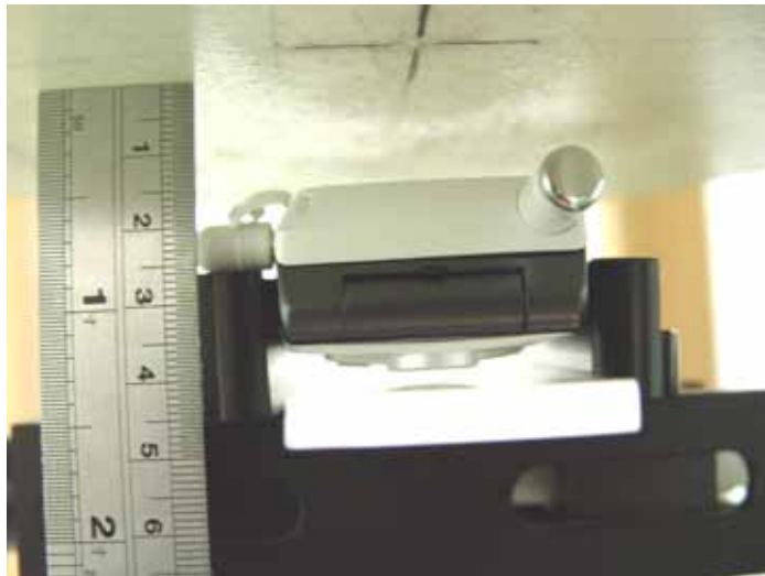
Fig. 8.8 Keypad Down with 1.5cm Gap
