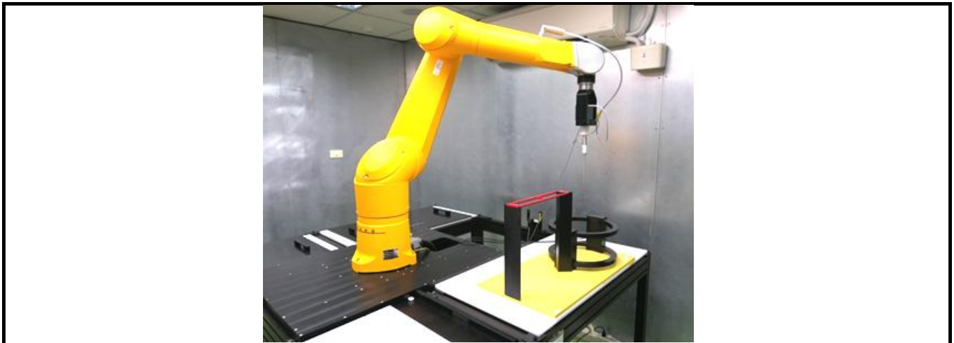
Fig-3.2 DASY52 Measurement System
