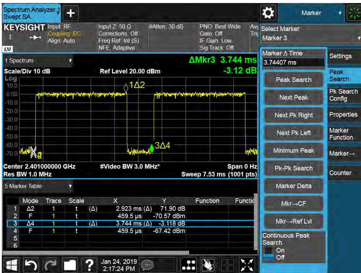
Time-domain plot for Bluetooth transmission signal
