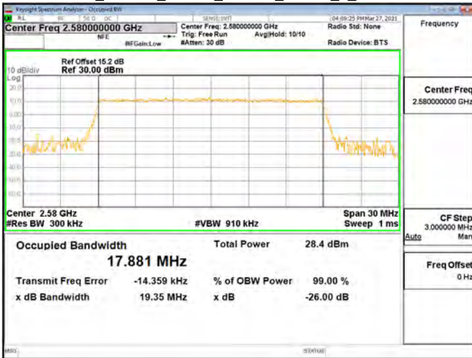
OBW_Band38_20MHz_64QAM_RB100_0_CH38000
