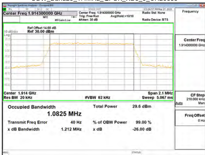
OBW Band25 1.4MHz QPSK RB6 0 CH26683
