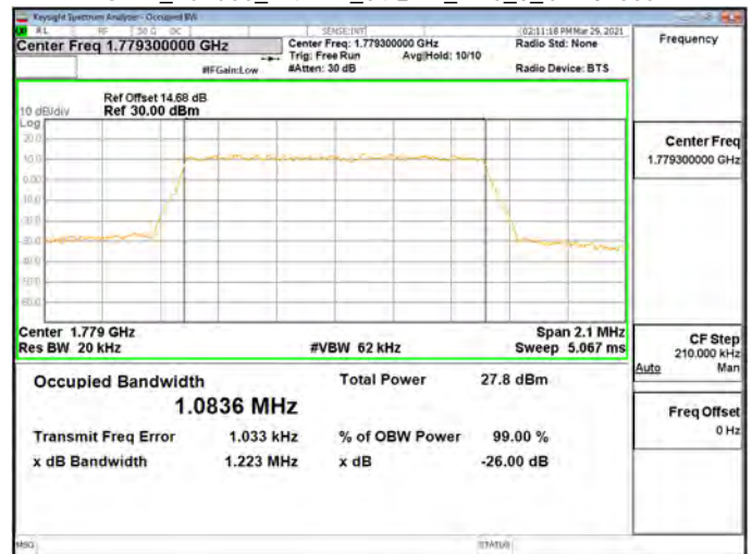
OBW_Band66_1.4MHz_64QAM_RB6_0_CH132665
