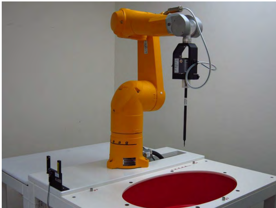
Fig.1 Photograph of the SAR measurement system
