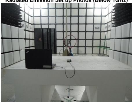
Radiated Emission Set up Photos (Below 1GHz)
