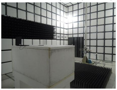
Radiated Emission Set up Photos (Front View)
