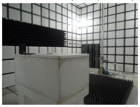
Radiated Emission Set up Photos (Front View)
