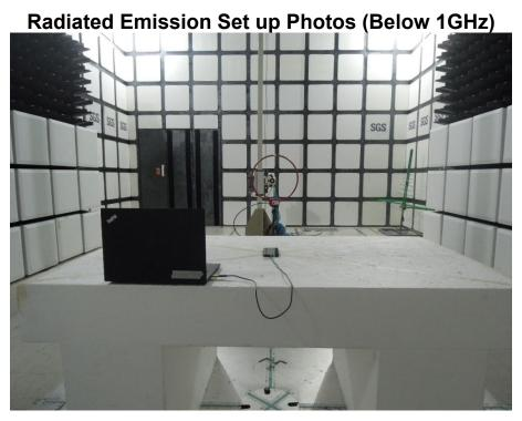
Radiated Emission Set up Photos (Below 1GHz)
