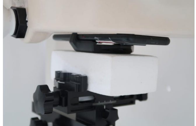
Front, Test Separation 0 mm _ AeroActive cooler
