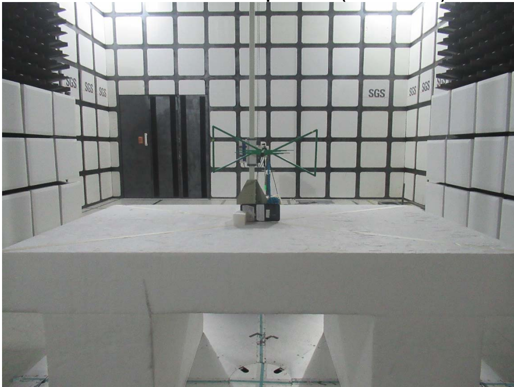
Radiated Emission Set up Photos (Above 1GHz)
