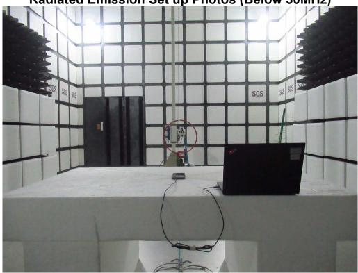
Radiated Emission Set up Photos (Below 1GHz)
