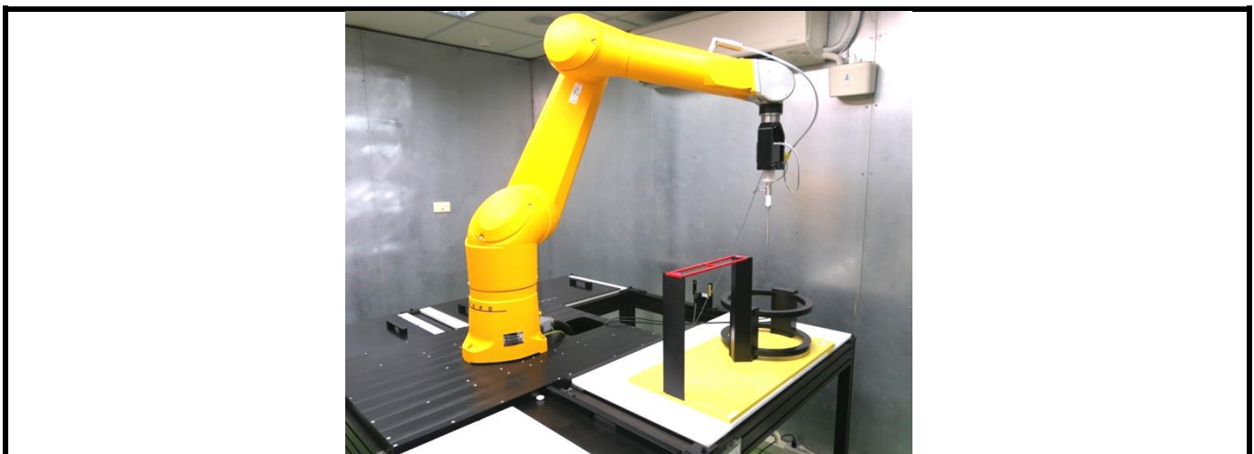
Fig-3.2 DASY6 Measurement System
