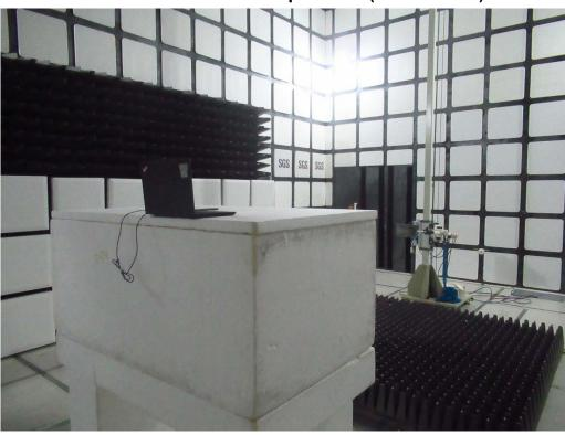
Radiated Emission Set up Photos (Above 1GHz)
