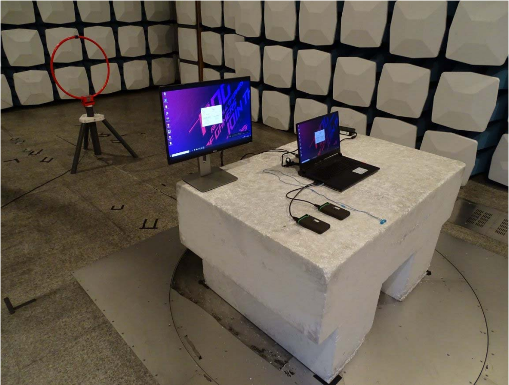
Front View of Radiated Test-LOOP
