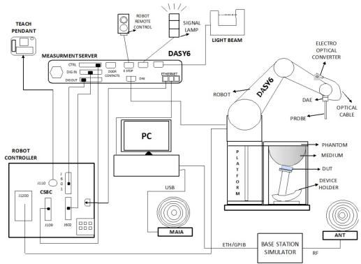
Fig-3.1 SPEAG DASY6 System Setup
