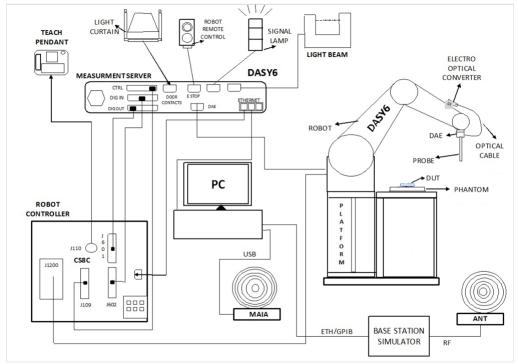
Fig-3.1 SPEAG DASY6 System Configuration
