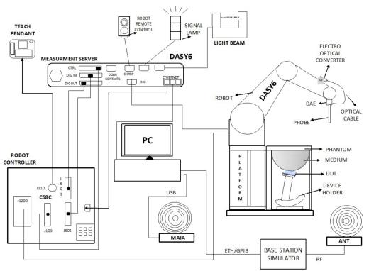
Fig-3.1 SPEAG DASY6 System Setup
