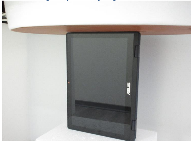
Testing Setup for Body, Right Side at 0 mm
