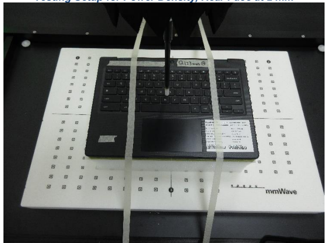
Testing Setup for Power Density, Rear Face at 2 mm
