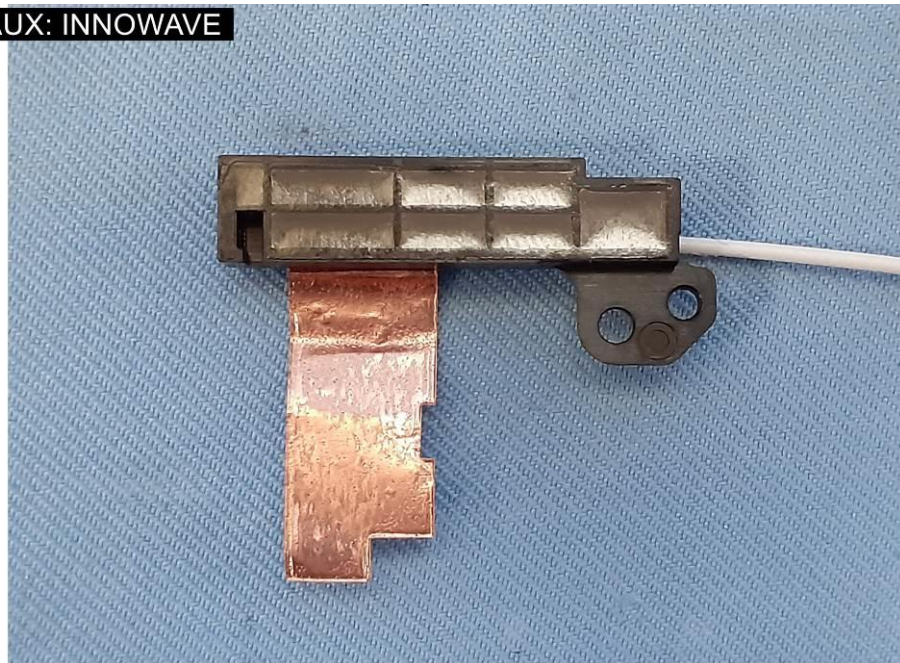
EUT Photo (40) WLAN antenna AUX : INNOWAVE
