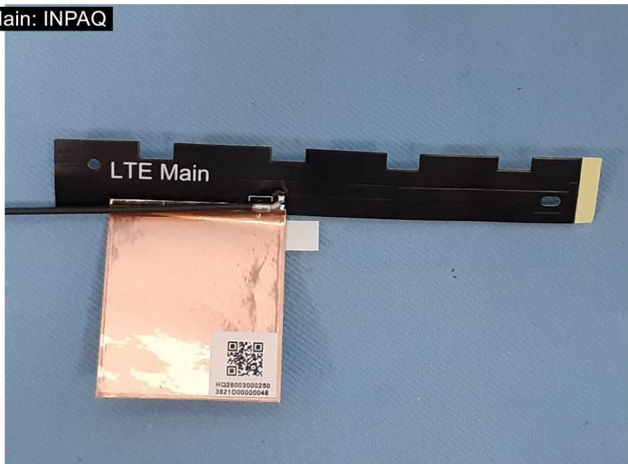
EUT Photo (26) WWAN antenna Main : INPAQ
