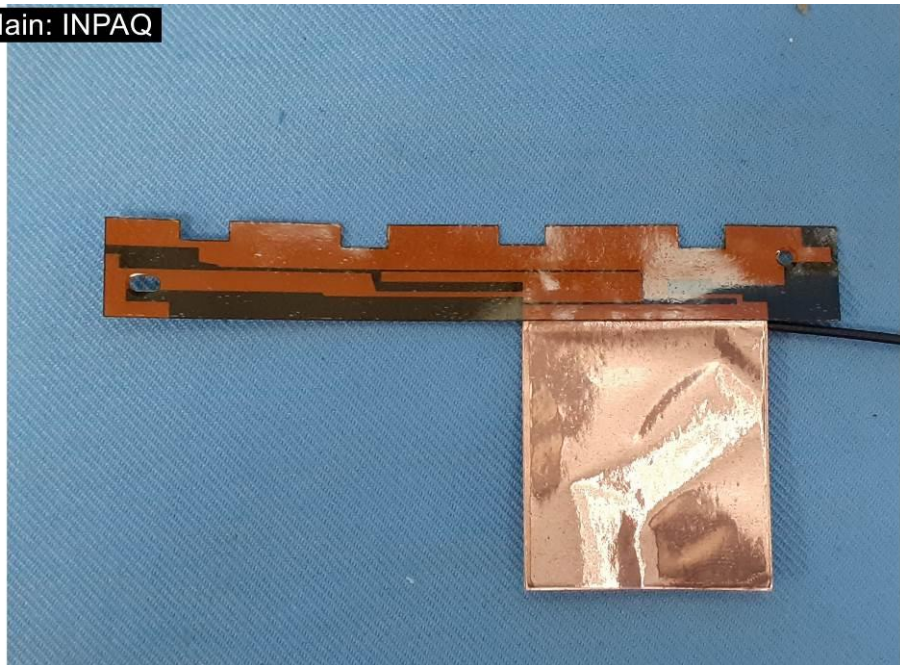
EUT Photo (28) WWAN antenna Main : INPAQ
