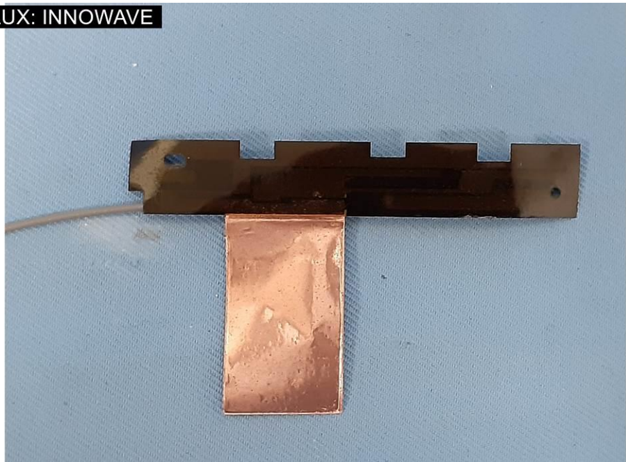
EUT Photo (48) WWAN antenna AUX : INNOWAVE
