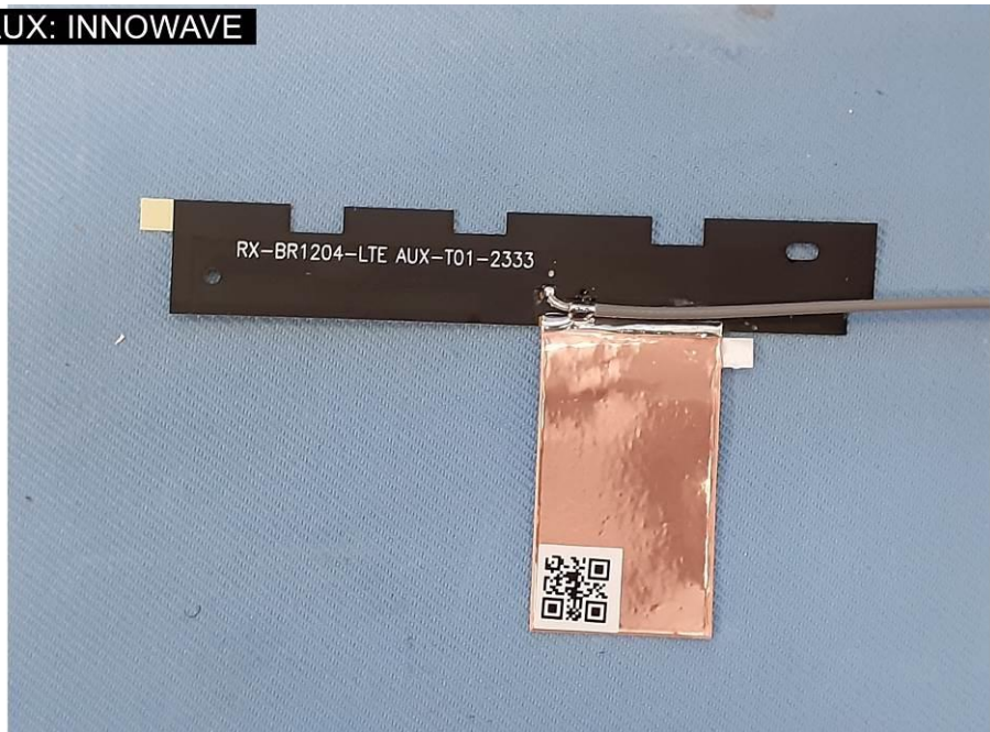
EUT Photo (46) WWAN antenna AUX : INNOWAVE
