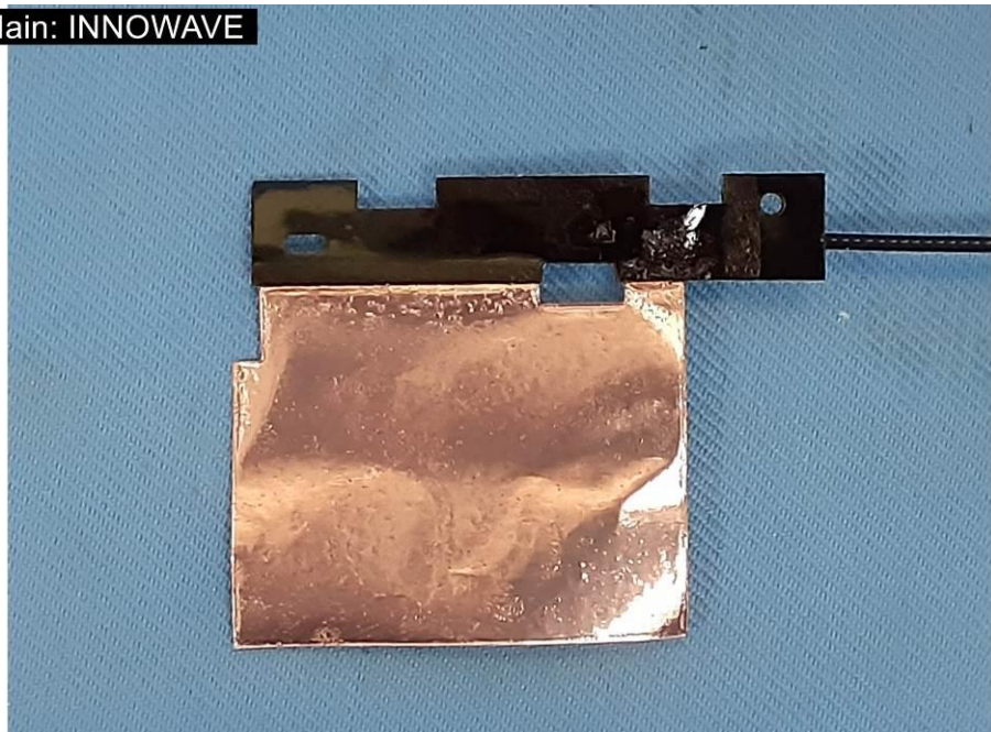
EUT Photo (36) WLAN antenna Main : INNOWAVE
