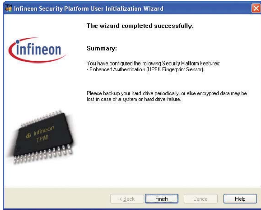
11. Settings are complete. Authentication when accessing TPM in Infineon Security Platform will change from asking TPM basic password to Biometric device (Fingerprint Reader) or new passphrase.
