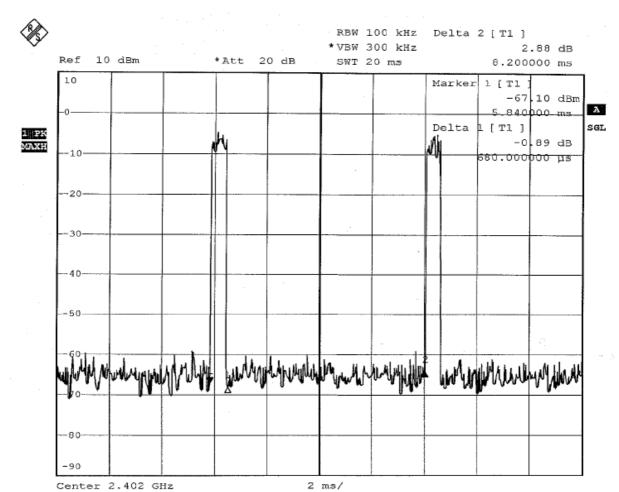
$$20\log(\text{Duty cycle}) = 20\log\frac{0.68 \text{ ms}}{8.2 \text{ ms}} = -21.62\text{dB}$$
