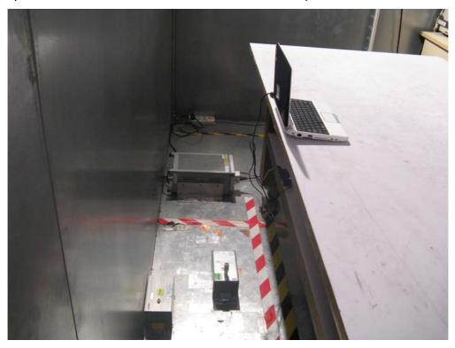
Test Mode: Mode 2: Transmit by 802.11g
