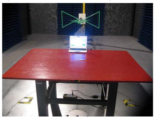
Test Mode : Mode 4: Transmit by 802.11n (40MHz Bandwidth)
