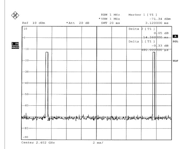
$$20\log(\text{Duty cycle}) = 20\log\frac{0.48 \text{ ms}}{14.36 \text{ ms}} = -29.51 \text{dB}$$
