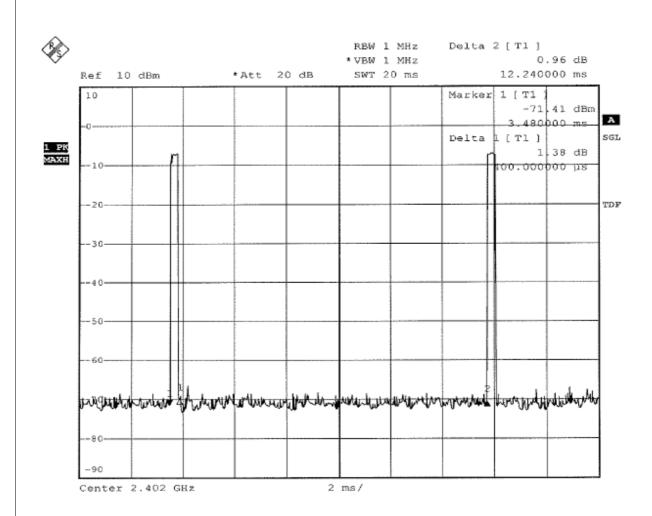
$$20\log(\text{Duty cycle}) = 20\log\frac{0.4 \text{ ms}}{12.24 \text{ ms}} = -29.71 \text{dB}$$
