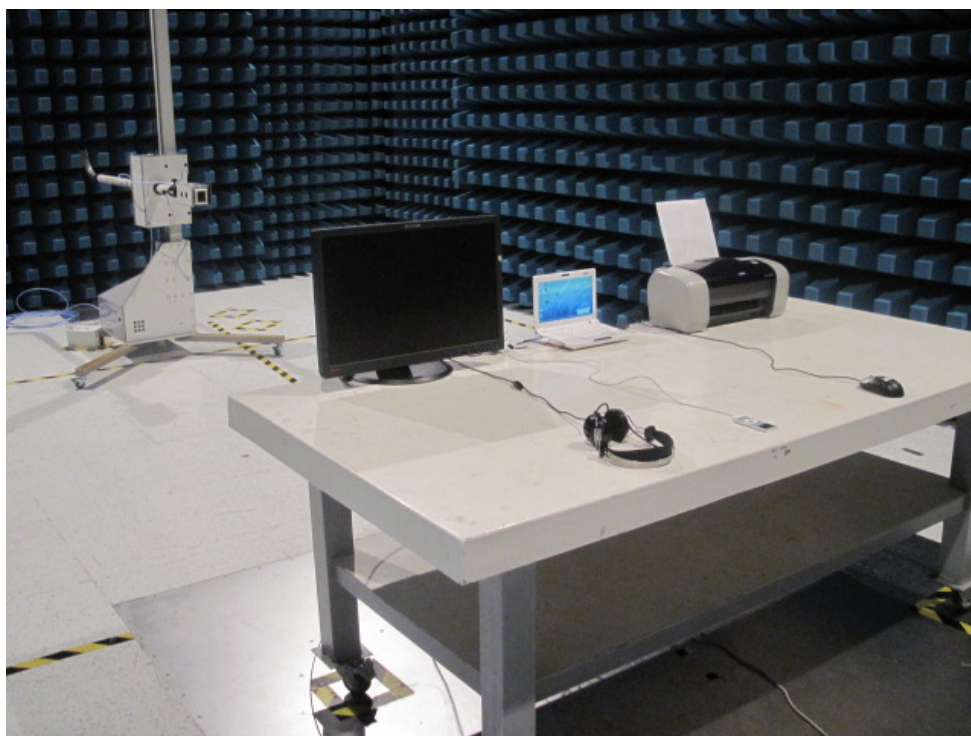
Description : Front View of Radiated Emission Test Setup for Above 18GHz
