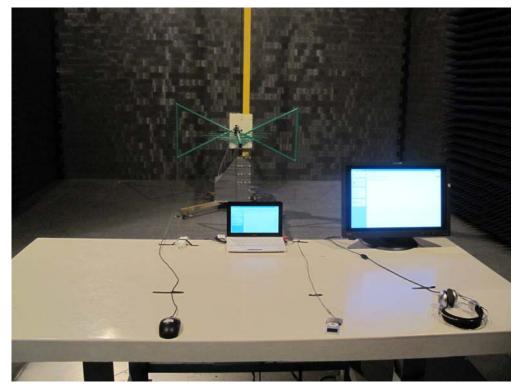
Test Mode : Transmitting Description : Front View of Radiated Emission Test Setup for 1~18GHz
