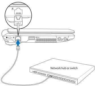
Network cable with RJ-45 connectors
