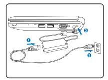
With the AC power cord connected to the AC-DC converter, connect the AC power cord to an AC outlet (preferably with surge-protection) and then connect the DC plug to the Eee PC. Connecting the AC-DC adapter to the AC outlet first allows you to test the AC outlet's power and the AC-DC converter itself for compatibility problems before connecting the DC power to the Eee PC. The power indicator on the adapter (if available) will light if the power is within accepted ranges.
