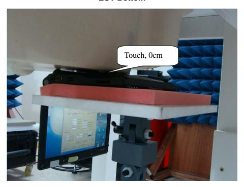
Note: The positions used in the measurements were according to IEEE 1528-2003.
