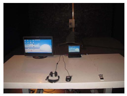
**SAR Test setup**
