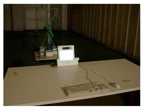
Front View of Radiated Test (above 30MHz)
