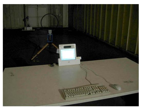
Front View of Radiated Test (below 30MHz)
