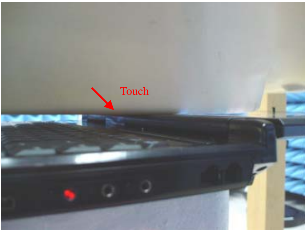
Fig.6 Photograph of the LCD Panel of Auxiliary Antenna contact to the flat phantom ; and at a distance of 0.0 cm from the base of the phantom
