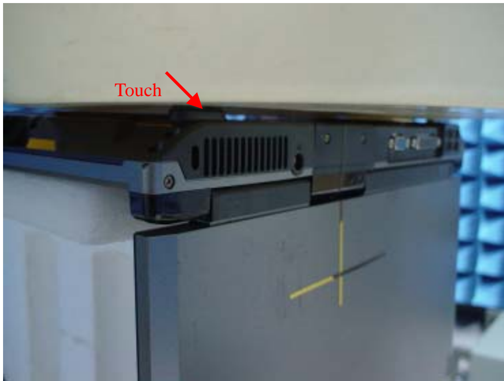
Fig.7 Photograph of the Bottom face of Auxiliary Antenna contact to the flat phantom; and at a distance of 0.0 cm from the base of the phantom.
