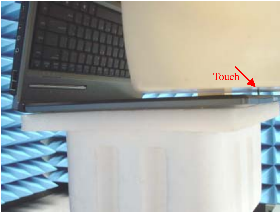
Fig.3 Photograph of the LCD Panel of Main Antenna contact to the flat phantom; and at a distance of 0.0 cm from the base of the phantom.
