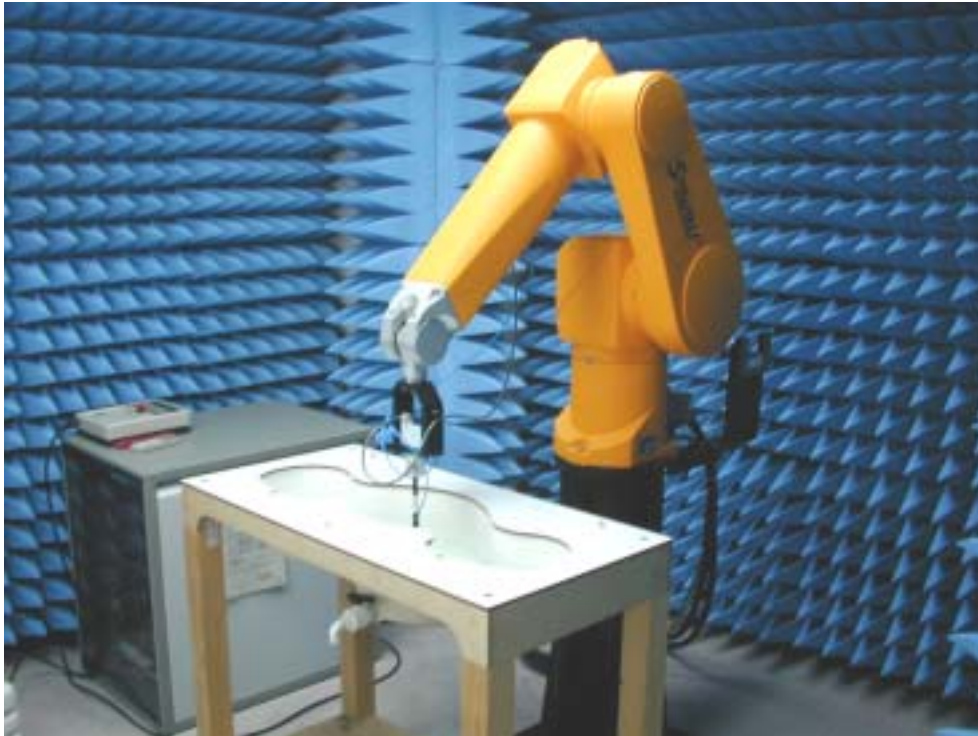
Fig.1 Photograph of the SAR measurement System
