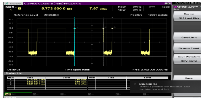
Time-domain Plot for Bluetooth Antenna-1 Transmission
