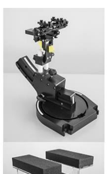
The DASY device holder is designed to cope with the different positions given in the standard. It has two scales for device rotation (with respect to the body axis) and device inclination (with respect to the line between the ear reference points). The rotation center for both scales is the ear reference point (ERP). Thus the device needs no repositioning when changing the angles.
