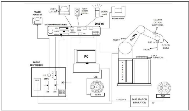
The DASY6 system for performing compliance tests consists of the following items:
