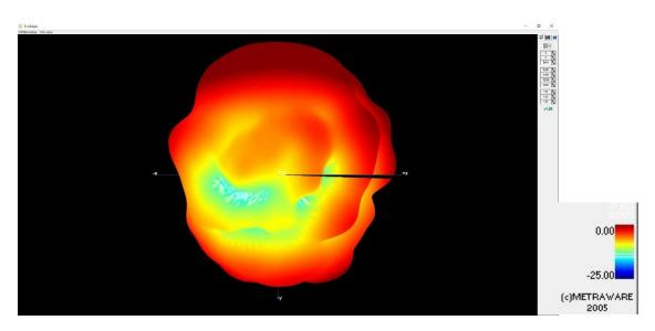
Max Antenna 3D Radiation Pattern 5150-5250 MHz
